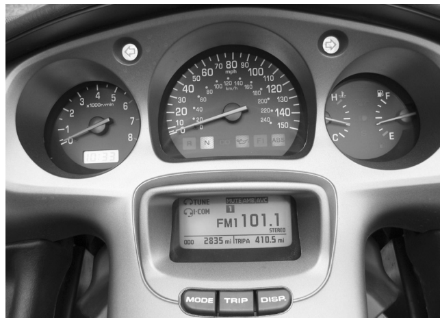
The Wing's highly-functional dash not only provides a lot of information, note how everything is well recessed and shaded from sun glare.
