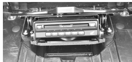
Top: The Honda's optional CD changer pops up out of the trunk floor for loading, then hides away, using up no packing space. Bottom: It may be the best-looking touring saddle in the world, and it's pretty darned good, but the LT's is even better.
