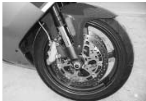
Above: Although not Aprilia's best, the "triple-bridge" Brembos and Showa fork were hard to fault. But its Michelin Pilots caused standup under braking.
