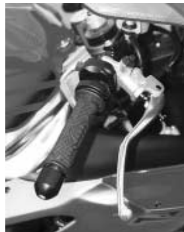
Below: The latest "radial pump" master cylinders are used on the clutch and brake for improved action.
