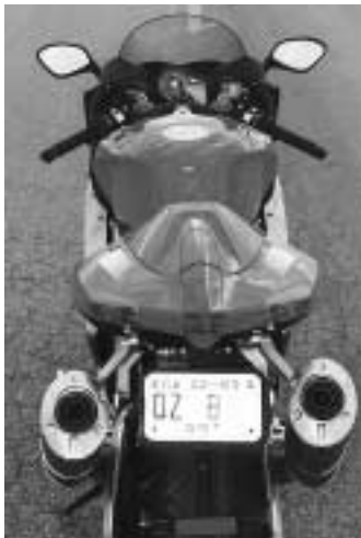
Above: The Mille's new shape is much narrower between the legs, and lower, too. Note new dual exhausts, integrated turnsignals and narrow mirrors.
