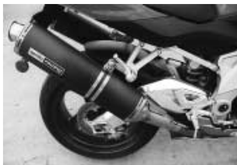
Above: Although not Aprilia's best, the "triple-bridge" Brembos and Showa fork were hard to fault. But its Michelin Pilots caused standup under braking.
